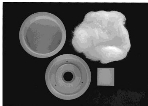
Figure 2. Components of the flow-through device: (upper row, from left to right) plastic bottom member and absorbent material; (lower row, from left to right) plastic top member and membrane.
